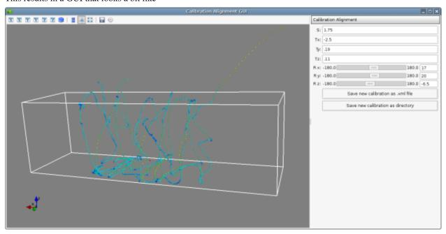
Using the controls on the right, align your data such that it corresponds with the 3D model loaded by STIMULUS.xml. When you are satisfied, click either of the save buttons to save your newly-aligned calibration.
