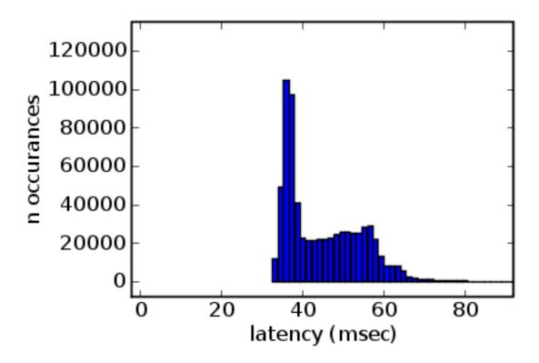
As of Feb. 20, 2008, the *LED\_test\_latency* script was used to test total latency from LED on to UDP packets with position information. This total latency was between 34-70 msec, with the 3D reconstruction latency being from about 25-45 msec. Note that these are from the initial onset of illumination, which may have different amounts of latencies than ongoing tracking.
